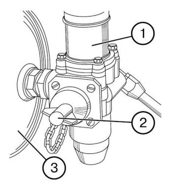
**IMPORTANT!** If pressure in a balloon exceeds 7,7 kgf/cm<sup>2</sup>, the compressor is switched over to idling by a pressure regulator and tires inflation stops automatically. Thus, control a pressure level by an indicator on the dashboard and decrease pressure through a condensate ejection valve if necessary.
