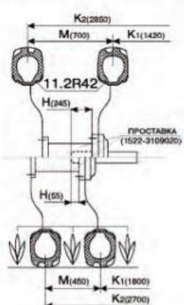
Sizes in brackets are given for inter-rows of 750 mm
